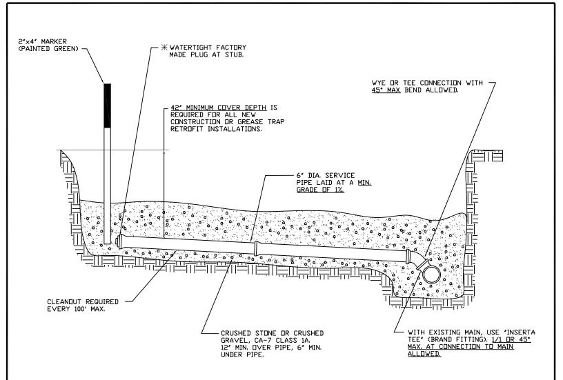
\* ALL BUILDING CONNECTIONS ARE REQUIRED TO BE OVERHEAD. STUBS AT THE RIGHT OF WAY SHALL BE CONSTRUCTED TO NO DEEPER THAN 6'-7'. WHERE CONFLICTS EXIST BETWEEN THE WATERMAIN (OR WATER SERVICES) AND SANITARY SERVICES, INSTALL SANITARY TO MAXIMUM DEPTH TO AVOID CONFLICT. IN THE EVENT OF CONFLICTS, REFER TO "77 ILL. ADMIN. CODE PART 890, ILLINDIS PLUMBING CODE", LATEST EDITION.
